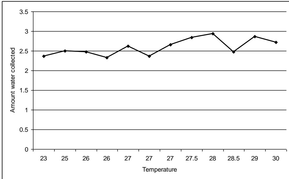
Figure 3. Amount of water [L/m<sup>2</sup>/day] collected in the Lowveld at different ambient temperatures [°C]
