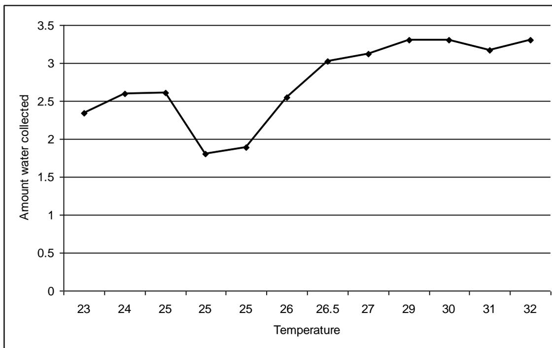
Figure 2. Amount of water [L/m<sup>2</sup>/day] collected in the Middleveld at different ambient temperatures [°C]
